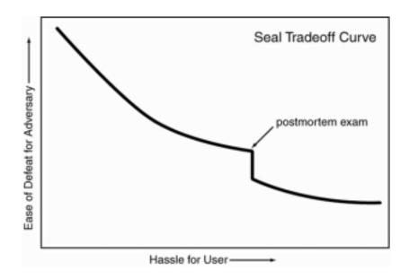
**Figure 2:** A schematic tradeoff curve for a typical seal. The more work the user puts into using the seal, the more difficult it is for an adversary to defeat it. The sharp dip in the curve is due to implementation of a postmortem exam after the seal is removed. Though the rest of the curve is drawn smoothly, a magnified view would typically show a series of small stair steps--each small drop representing the introduction of a new procedure into the seal protocol.
