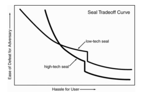
Figure 3: Typical tradeoff curves for low-tech vs. high-tech seals (including seals that use high-tech readers). While the high-tech seal can provide better tamper-detection, you often must actually do more work, not less, to achieve the higher security.
